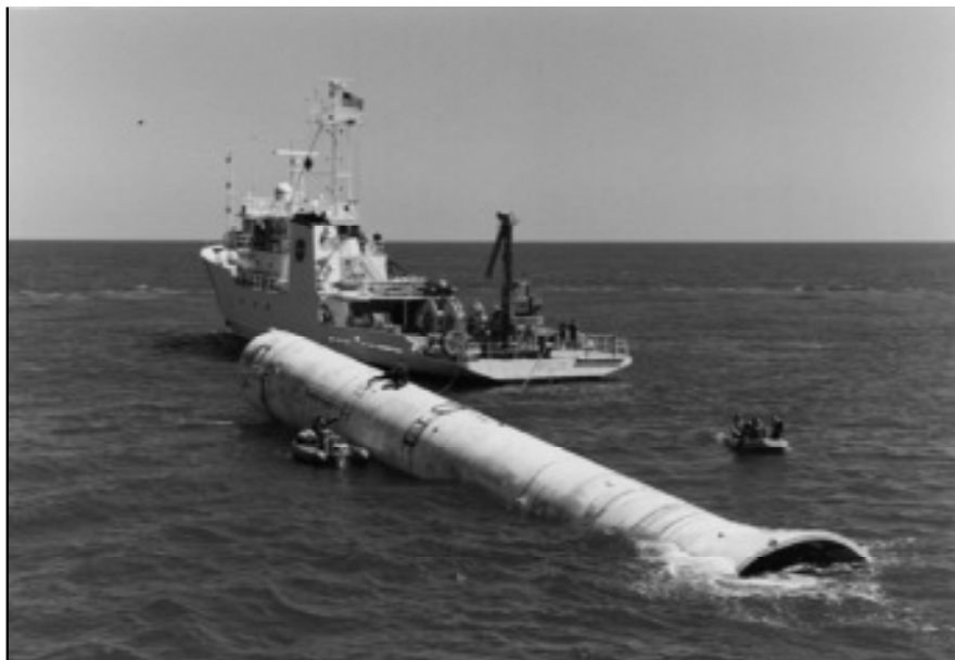
A TEAM from the U.S. Army Explosive Ordnance Disposal Unit at Cape Canaveral Air Station sets six charges to be detonated by remote control on the Ocean Test Fixture (OTF). The Liberty Star, which towed the OTF to sea, is in the background.
