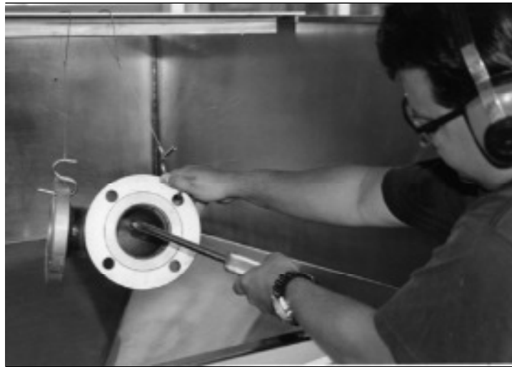
I-NET, Inc. technician Chris Fogerty cleans a stainless steel gaseous oxygen valve with the Supersonic Gas-Liquid Cleaning System in the Engineering Support Building at Complex 34 on Cape Canaveral Air Station. The minute amounts of water used by the system are captured in the cleaning hood of the unit for analysis.
